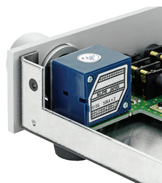
A key component of the Drachenfels is its volume control - an expensive ALPS dual pot.
